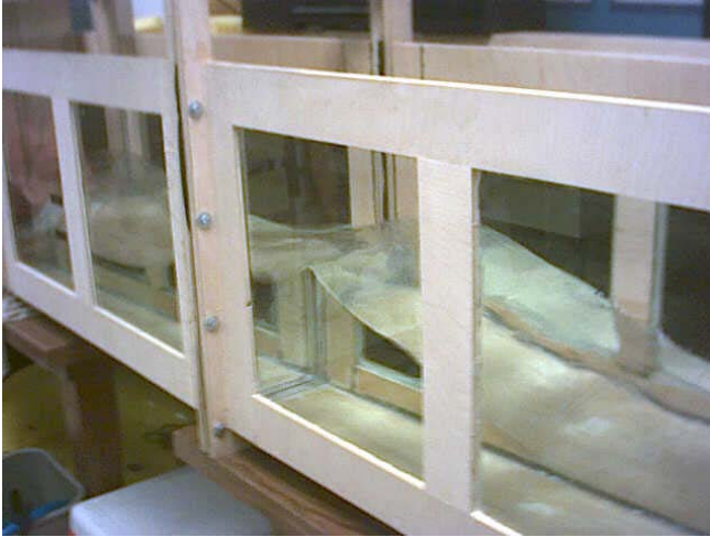
Water wave generation tank in the Department of Marine and Environmental Systems (built by Dr. Eric Thoeston) in the Physical Oceanography lab at Florida Tech.
