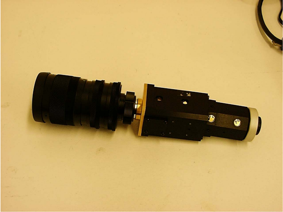
The above image shows a lens coupled to an imaging spectrograph made by SPECIM in Finland.
