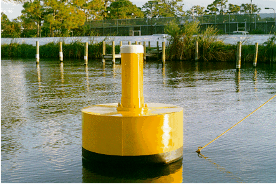
Shallow water hyperspectral optical buoy for measuring water quality parameters. Utilizes an active or passive sensor design patents owned by KB Sciences in Beaufort, South Carolina.
