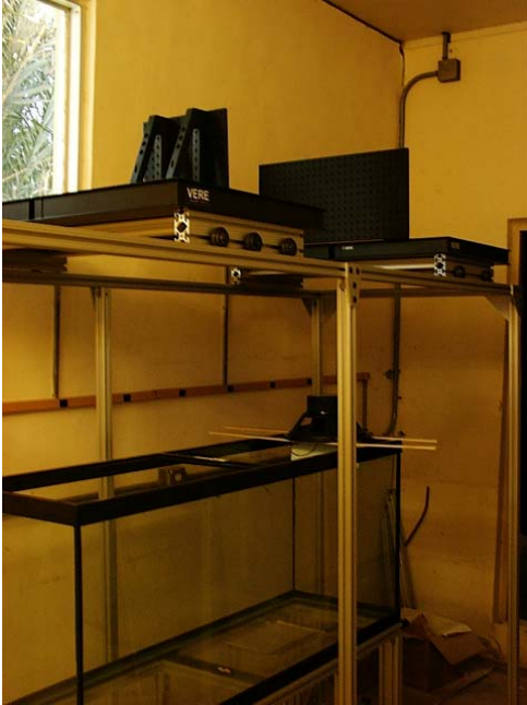
Laboratory system for mounting camera, spectrograph and laser system over a small water tank for imaging submerged features and capillary water waves generated from an acoustic water wave generator being built by Dr. Bostater in the Environmental Optics Lab at Florida Tech.
